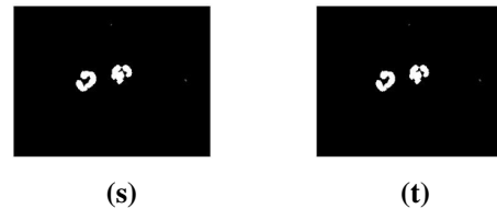
Figure10: (s)Regional maxima superimposed on original image(I2), (t)Modified maxima superimposed on original image(rgm4).
